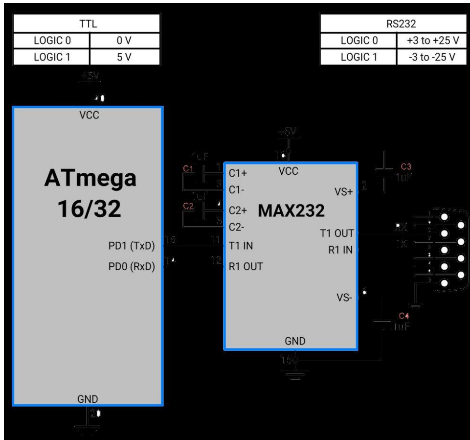
ATmega16/32 Serial Interface Connection Diagram
